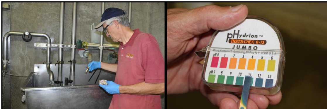
Figure 3. Check that the pH of the detergent solution is between 11 and 13. Remember to use safety equipment (gloves and goggles) to protect from splashing.
