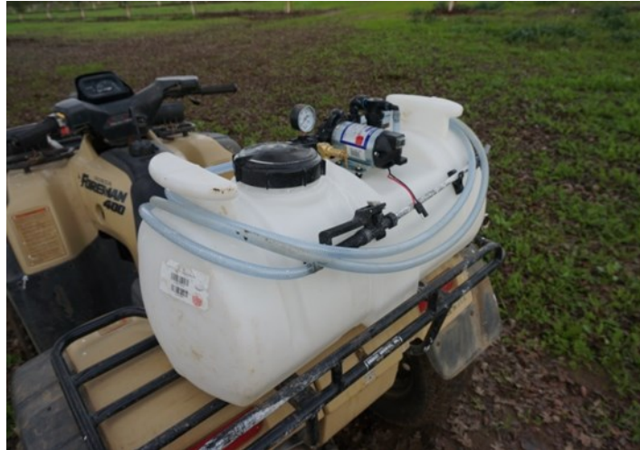
Figure 3. 15 gallon spray tank with electric pump mounted on an ATV to deliver 50/50 interior latex paint/water mix quickly.
